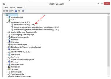
Please note that the number of a COM port must not be assigned twice. If necessary, change the associated COM port number in the device manager.
