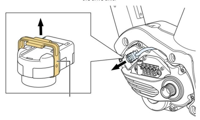
The speed sensor which is plugged into the rearmost (right) socket can remain connected to the drive unit and does not need to be removed.
