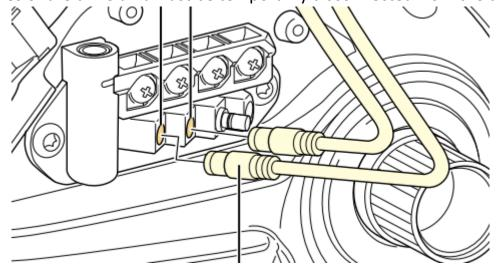
In addition, the big front facing left battery connector on the drive unit must also be temporarily disconnected. To do this, pull the handle out of the plug to make it easier to remove the plug from the drive unit:
