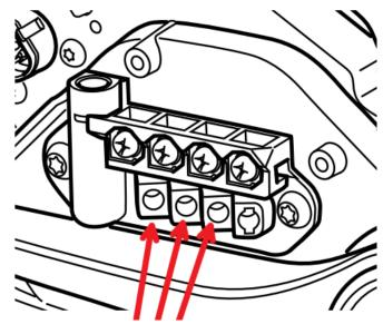
When connecting the battery connector, make sure that it is pushed on carefully and straight so as not to bend any contacts:
