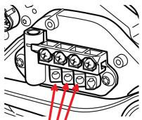
Please ensure that all necessary cables of the Shimano STePS bus system are correctly inserted (and locked with a "click" - feeling) into the corresponding receptacles. Ideally use the TL-EW300 tool for this. Please do not use pliers or similar tools to insert or remove the plug connectors as these could damage the sensitive cables or plugs! If you don't have a special tool, then insert or remove the plug carefully with 2 fingers. Please do not pull on the cables as this could damage the cables!
